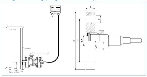
The standard transducer is supplied with DN25, DN40 or DN50 PN16 DIN2527 flange manufactured of ASTM 316L steel.
